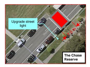
This Speed Hump will be 75mm high and 6 metres long with a 1.5 metre ramp on each approach.
