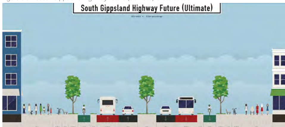
Figure 6.5: South Gippsland Highway Future (Ultimate) Cross-Section
