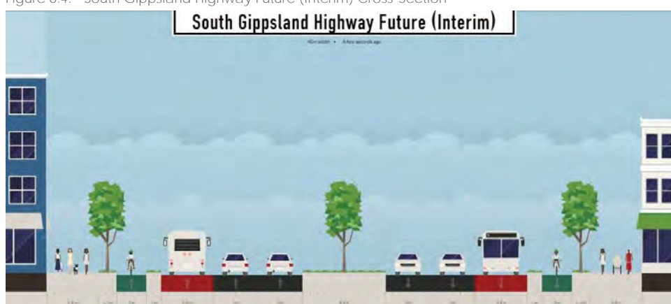
Figure 6.4: South Gippsland Highway Future (Interim) Cross-Section
